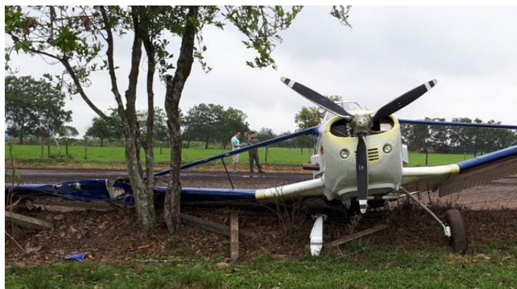
Image No. 4 - Agricultural aviation accident due to loss of control on the ground (LOC-G)
